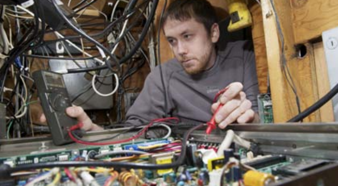
Field electronics technician Jeff McMahon checks components on a radar amplifier located inside the helm's control cabinet.
