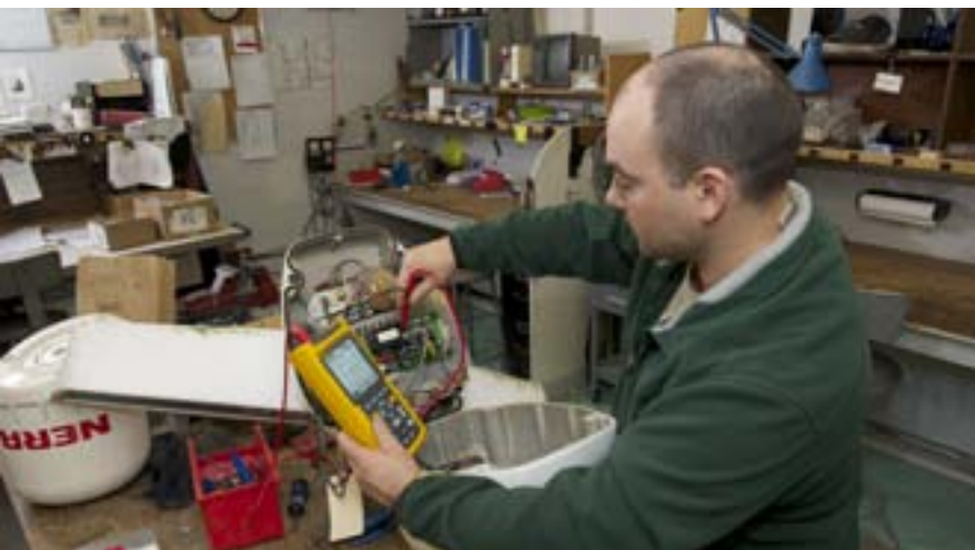
Trevor Comstock checks the magnetron current on a radar antenna unit.
