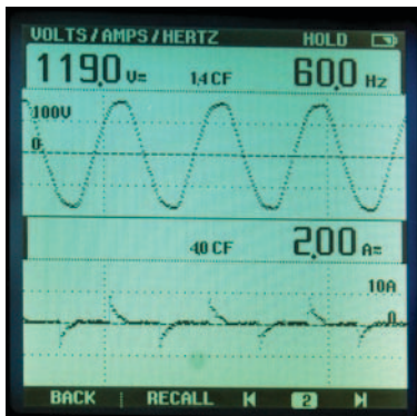
CFL current harmonics. There is 76 % total harmonic distortion (THD) in this current. The total harmonic current reading (1.77 A) is much greater than the fundamental 60 Hz current (1.15 A). The graph shows that harmonics up to the 51st (3,060 Hz) are present due to the nonlinear current flow.
