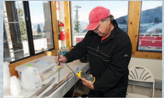
As Ted Bartkoski demonstrates, temperature readings start by testing the reference runner at room temperature early in the day.
