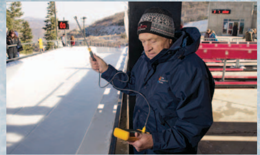
A veteran official at Olympic events, Don Banford checks and records ice and air temperatures using the Fluke 52 Series II Contact Thermometer and 80PK-27 Surface Temperature Probe.
