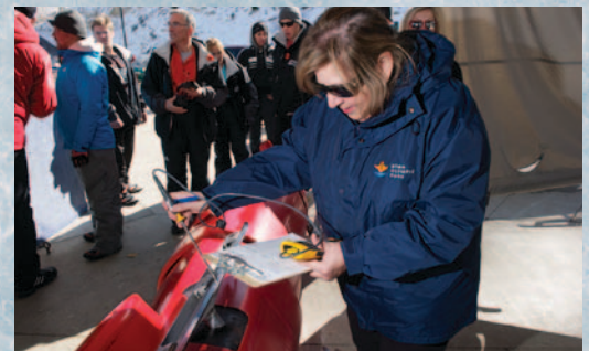
Using the Fluke 52 Series II Contact Thermometer and 80PK-27 Surface Temperature Probe, Sue Kapis measures the reference runner temperature.
