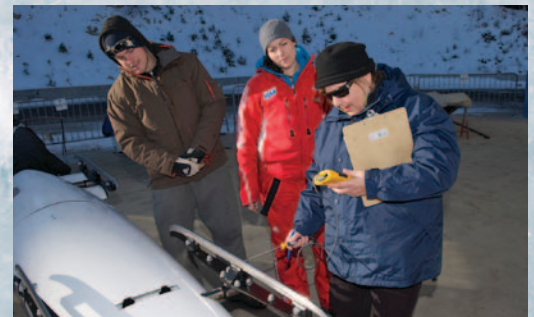
Sled runner temperatures must closely match those of a standard reference runner.
