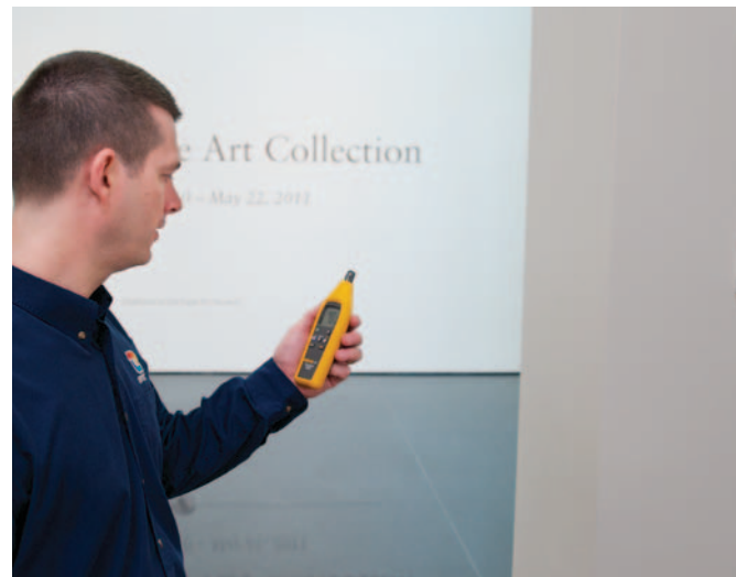
Mark Janco, System Specialist for ENTEC, uses a Fluke 971 to confirm that the temperature and humidity are at the optimum levels for a high-end art display.
