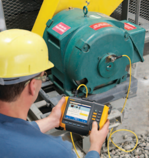
Vibration analysis measures the frequency and intensity of vibrations caused by wear, misalignment, looseness, and other mechanical problems.
