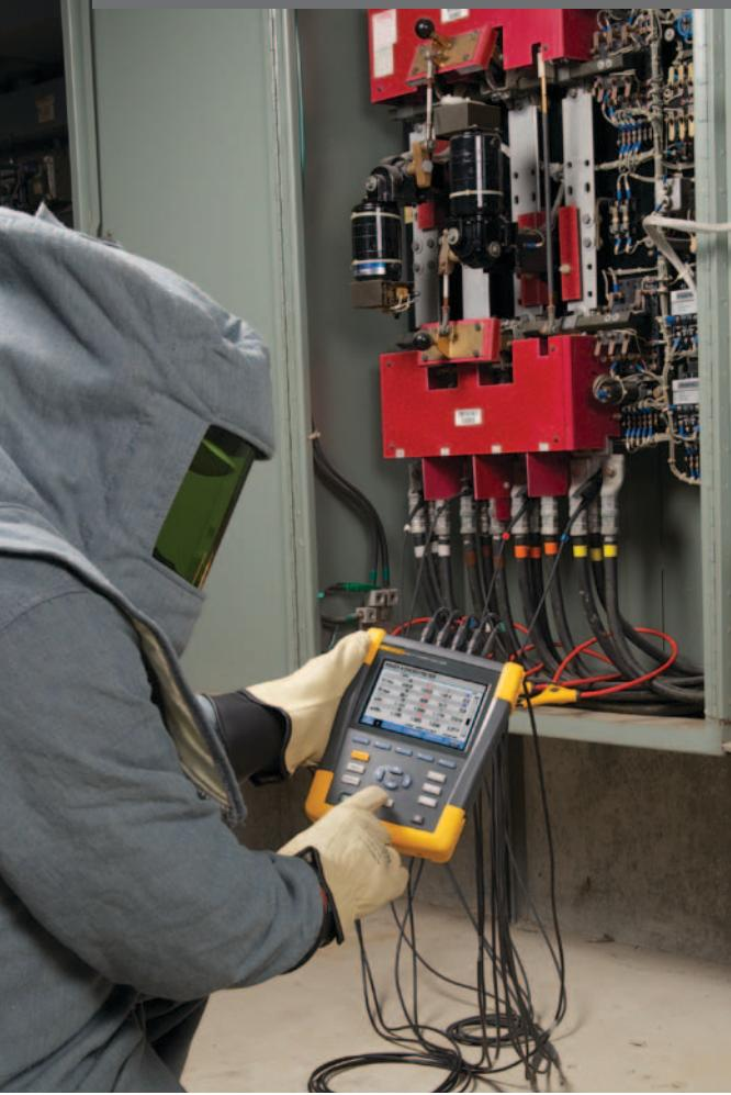
Use the Unified Power measurement feature and the Energy Loss Calculator on the new Fluke 430 Series II Power Quality Analyzers to determine how much power is affected by harmonics and load unbalance.
