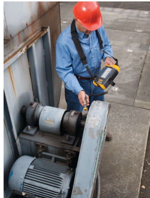
While vibration can be normal in machine operation, it can also be both a sign and a source of trouble. The hand-held Fluke 810 Vibration Tester is designed and programmed to diagnose the most common mechanical problems of imbalance, looseness, misalignment, and bearing faults.
