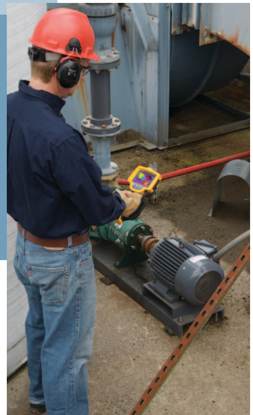
Rising heat becomes visible with a Fluke Ti32 Thermal Imager, which captures two-dimensional images of the apparent surface temperatures of pumps and other equipment.
