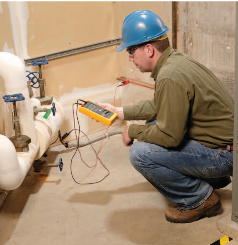
The Fluke 1621 Earth Ground Tester is an easy-to-use earth ground tester, the first line of defense in detecting reliable ground connections.
