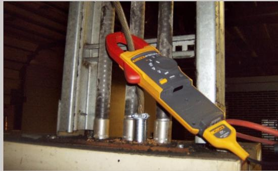
Using the Fluke 381 clamp meter, technicians measured a significant amount of ground current flowing from each air compressor. Photo courtesy of Linamar Corporation
