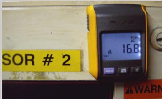
The Fluke 381 clamp meter's remote display attached to compressor #2 provided easy monitoring from several feet away. Photo courtesy of Linamar Corporation
