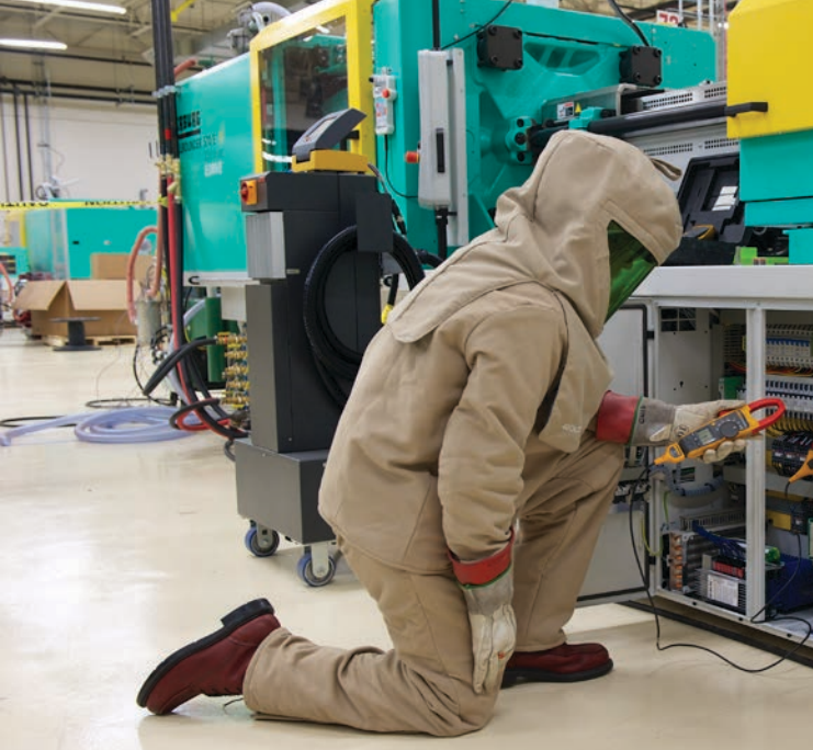
In the high-power environment of a plastic injection molding plant, Chipper Stohl uses his Fluke clamp meter and iFlex™ flexible current probe to check the current draw on a newly installed 200-ton plastic mold machine.
