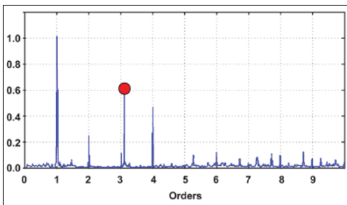
3. Increased non-synchronous peak.
