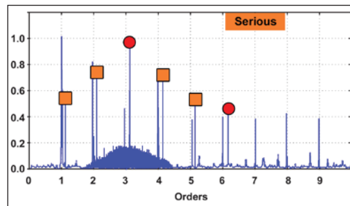
7. Noise hump near bearing tone.
