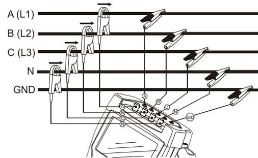
**Figure 1. Connection of Analyzer to 3-phase distribution system**
