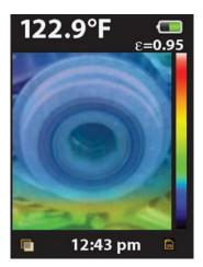
Normally functioning pulley.
