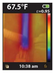
Normally functioning A/C orifice.
