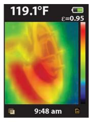
Typical heat generated from the brake rotor.
