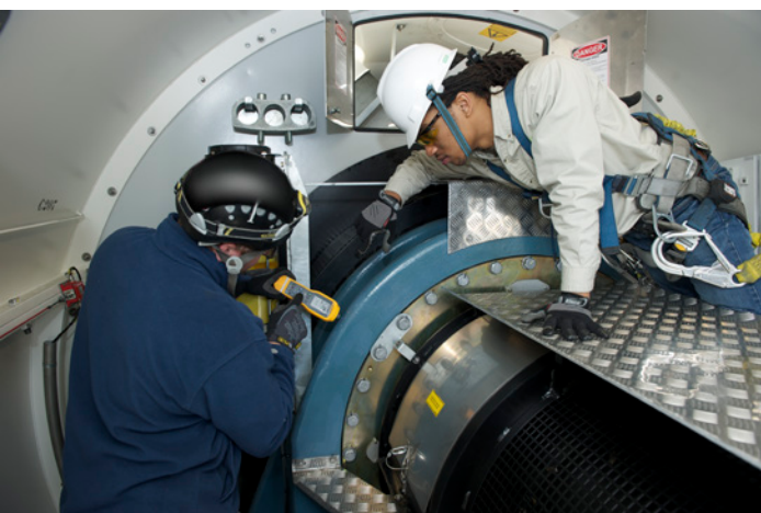
Jonathan Townsend looks on as a main bearing vibration is checked with the Fluke 805 Vibration Meter.
