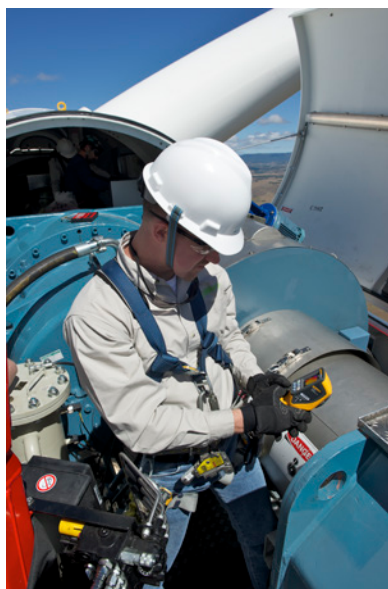
Jonathan Townsend looks on as a main bearing vibration is checked with the Fluke 805 Vibration Meter.
