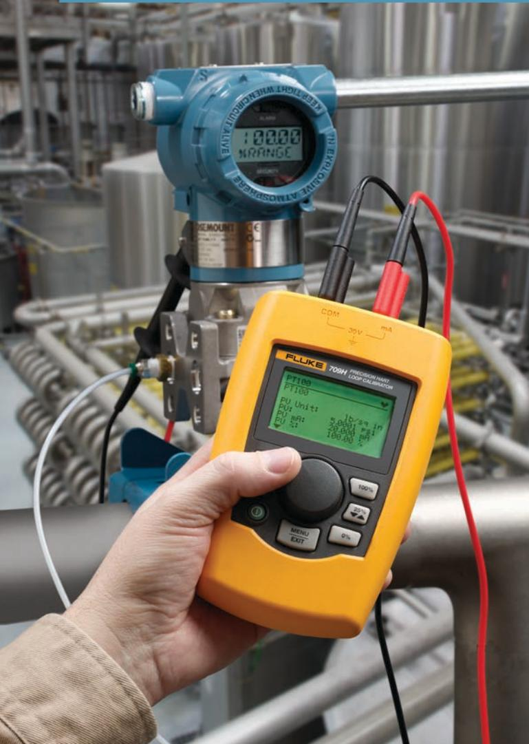
The Fluke 709H Precision Loop Calibrator with HART Communications/Diagnostics was built to be used with one hand; you can scroll quickly through menu options with the central dial.
