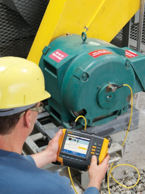
Vibration analysis on a fan motor, with the Fluke 810 Handheld Vibration Tester.
