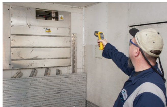
The external refrigeration unit might seem to be running correctly, but the output of the unit needs to be sufficiently cold. Brad uses a Fluke 561 Infrared and Contact Thermometer to check temperature.
