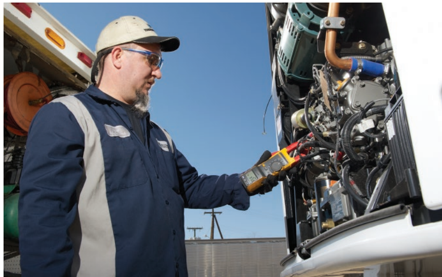
McCubbin uses a Fluke 381 Clamp Meter to check the starter cranking current, the health of the starter, and the on-board battery system. The Hazard-Risk Category of this setup is 0.
