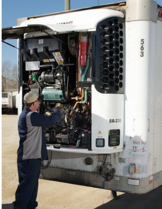
Brad McCubbin uses his Fluke 561 thermometer to check the running temperatures of the internal components of a Thermo King refrigeration unit mounted on a 53-foot (16-meter) tractor trailer. The Hazard-Risk Category of this setup is 0.
