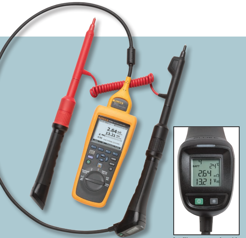
Intelligent test probe with integrated LCD display
