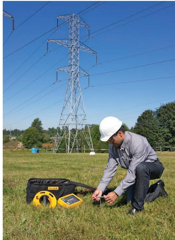
For the 3-pole Fall-of-Potential test, two earth stakes are placed in the soil in a direct line—away from the earth electrode.
