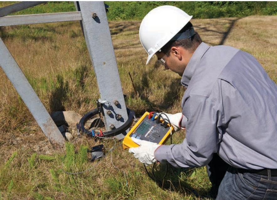
**Stakeless** measurement is possible by measuring earth ground loop resistances for multi-grounded systems using only current clamps. This test technique eliminates the dangerous and time-consuming activity of disconnecting parallel grounds, as well as finding suitable locations for auxiliary ground stakes. You can also perform earth ground tests in places you might not have considered before: inside buildings, on power pylons, or anywhere you don't have access to soil.
