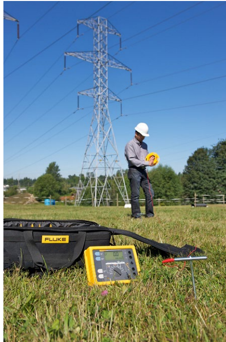
All required earth ground tests can be performed with the Fluke 1625-2 KIT
