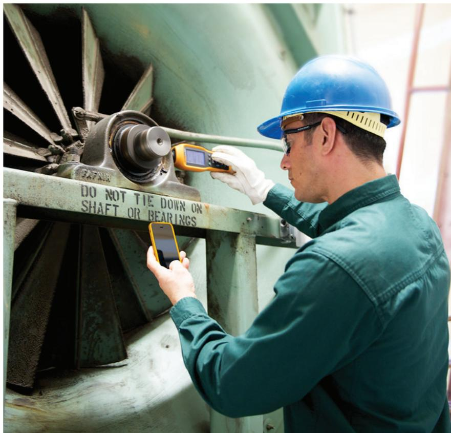
Instead of complicated vibration analyzers that require an experienced vibration expert to analyze complex waveform data, the vibration meter is a tool that a maintenance technician with no formal vibration analysis training can use to screen the many machines in the plant. The Fluke 805 FC quickly screens vibration in order to let the user know which machines are healthy and which ones need repairs.
