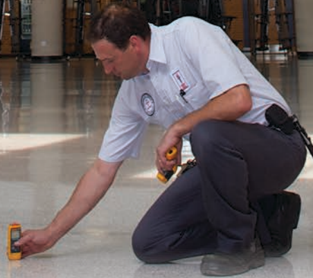
Measuring the area of a space with a laser distance meter, then taking ambient and vent temperature readings, helps ensure the HVAC system is performing correctly.
