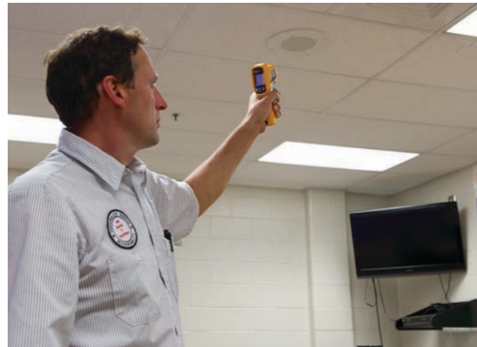
Each classroom needs to be comfortable. Here Mark uses his infrared thermometer to check ceiling vents.
