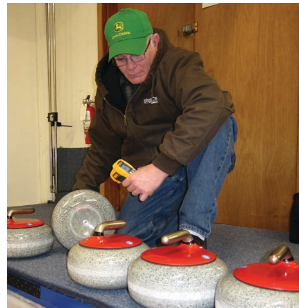
Dave Staveteig, head ice technician for USA Curling, uses the Fluke 62 Infrared Thermometer to check the temperature of a curling stone. Temperature is critical in the interaction between ice and the granite stones.
