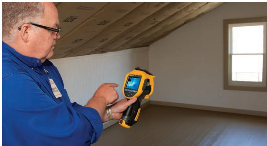
An expanse of wall might look uniform, but an infrared camera can detect temperature anomalies.
