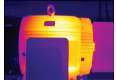
Overheating is one of the biggest factors in shortening that life. Operating at a temperature of  $\sim 10^\circ$  over its rated value can cut in half the service life of a motor. Therefore, regularly checking motor operating temperature is crucial to ensuring reliable operation of production systems.
