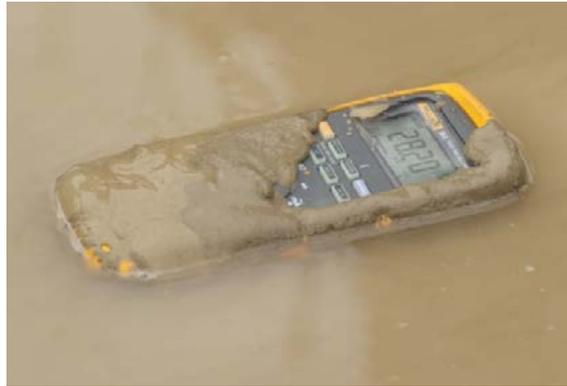
An IP67 rated-meter like the Fluke 28-II is better suited for outdoor work environments than meters rated for generic use.
