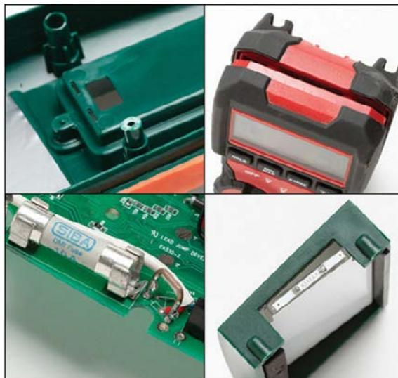
Damage to multimeters subjected to a six-foot drop onto concrete. Clockwise from top left: Broken screw boss, case separation, dislodged display, bent fuse clip with loose
