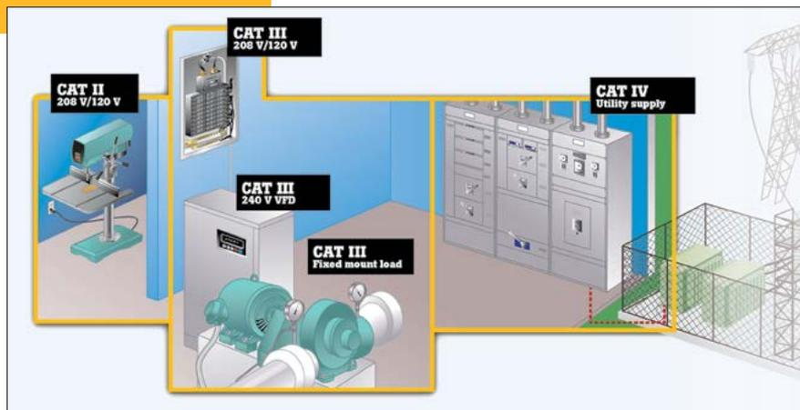
The IEC “CAT” rating is a combination of proximity to source and level of potential energy
