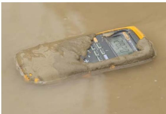
An IP67 rated-meter like the Fluke 28-II is better suited for outdoor work environments than meters rated for generic use.
