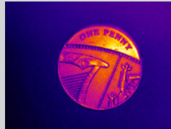
Figure 6. This penny, approximately 20.3 mm in diameter, was captured with a TiX560 camera and a standard lens.
