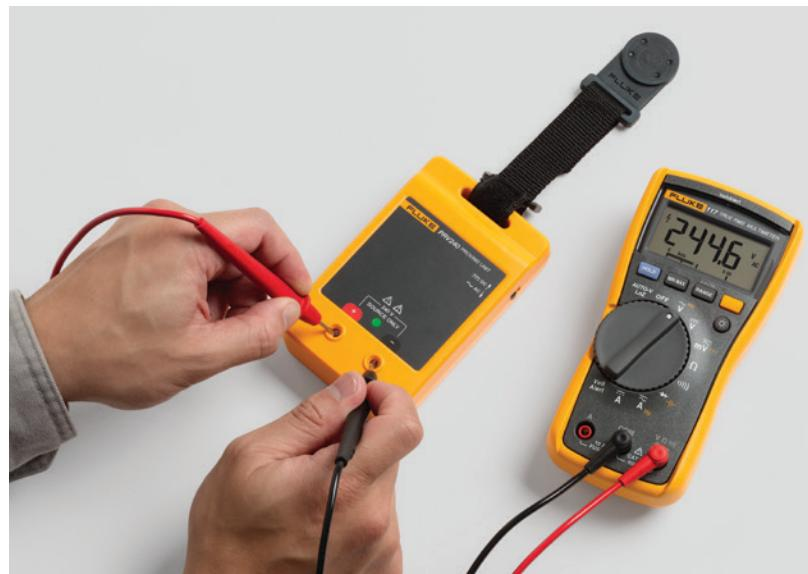
3. Check the voltage output of the PRV240 to ensure it has the verified voltage of 240 V  $\pm$  10 %. If the voltage output is not within limits as specified by Fluke Corporation, replace all the batteries and re-verify the voltage output of the PRV240. If the voltage output is within specified limits, the PRV240 is ready for field use.
