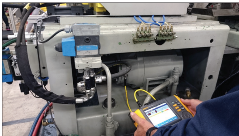
With the Fluke 810 Vibration Tester, know within a few minutes, the specific fault diagnosis, severity, and repair recommendations.
