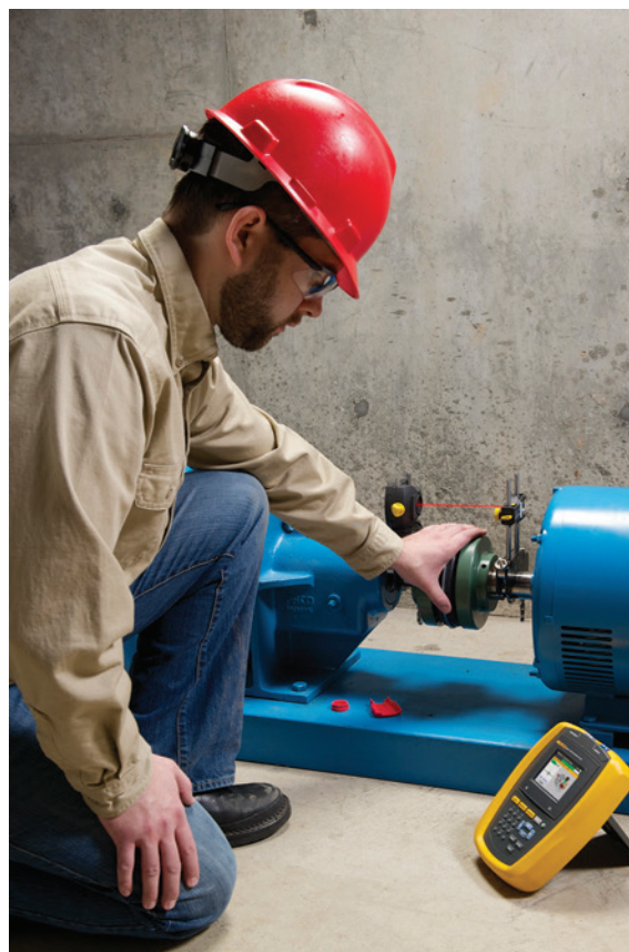
The Fluke 830 is an easy-to-use tool designed specifically for precision shaft alignment. It doesn't require extensive alignment education.
