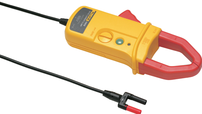
A multimeter accessory such as the Fluke i1010, 1000 A AC/DC Current Clamp will make a 10 A measurement without introducing significant burden voltage, and without breaking the circuit
