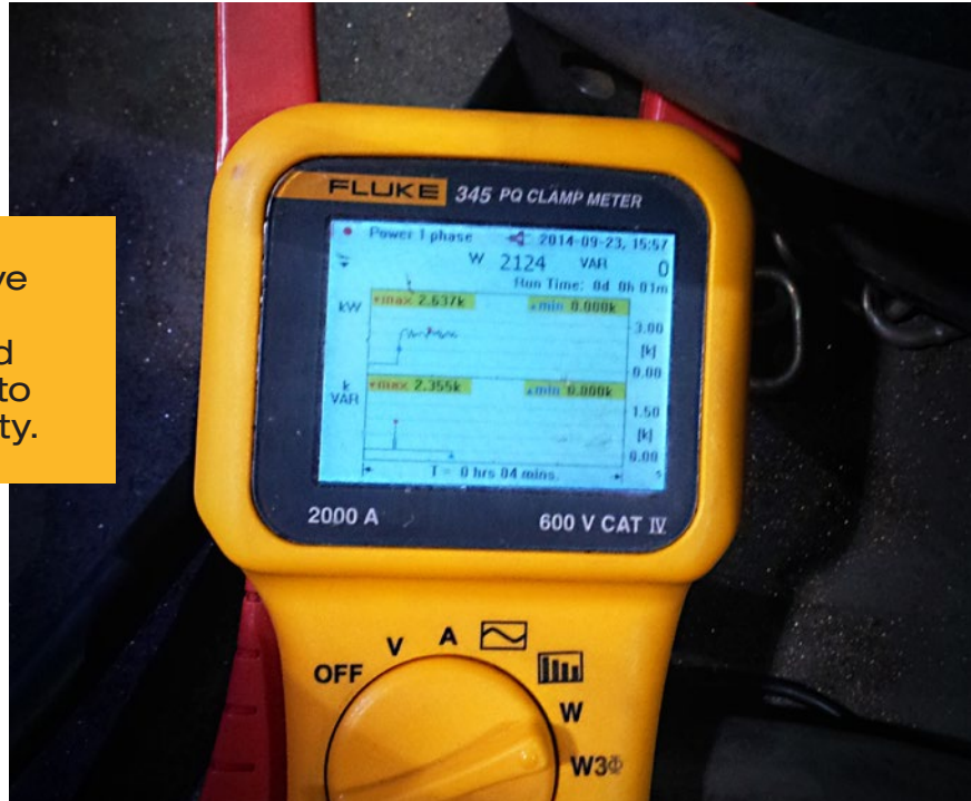
With the Fluke 345 set to read Single-phase watts, the heat input applied to a given length of weld can be determined.
