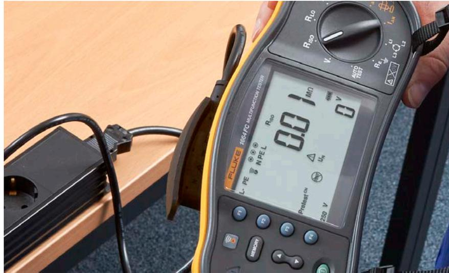
If the tester detects that an appliance is connected, it will stop the insulation test and provide a visual warning. This helps eliminate accidental damage to peripheral equipment and keeps your customers happy.
