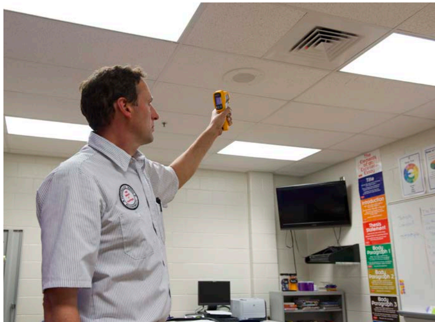
Mark checks discharge air temperatures in classroom registers with his 62 MAX
