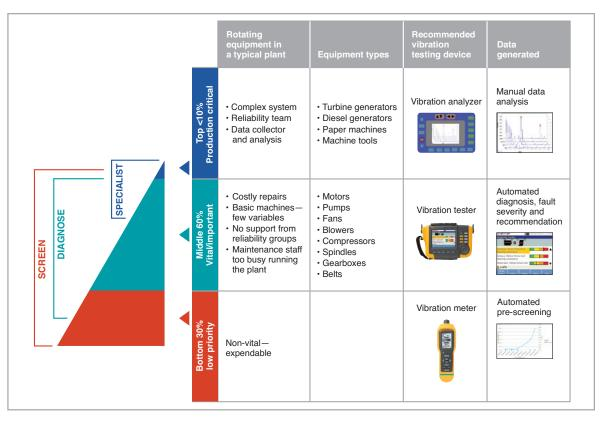
Finally, refer "any few" remaining complex faults "(less than 10% of faults)" to an expert consultant with an **analyzer**.
