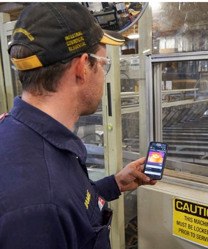
their smartphones, using the ShareLive™ function on the Fluke Connect app. This allows all the team members to see the same set of measurements on their smartphones as they activate and deactivate the machines on the line. They can isolate individual devices and check voltages until they finally narrow down the anomaly.
