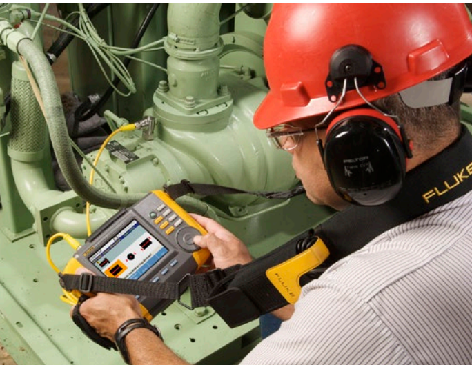
The award-winning Fluke 810 Vibration Meter uses an auto-diagnostic program that helps workers stay efficient.
