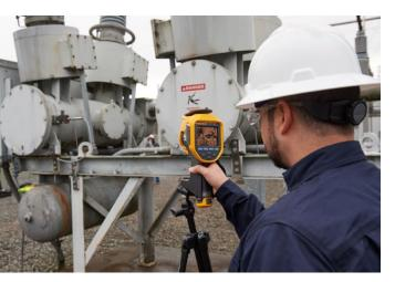
Figure 1. An inspector uses the Fluke Ti450 SF6 Gas Detector to inspect bolted connections.
