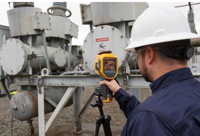
Figure 1. An inspector uses the Fluke Ti450 SF6 Gas Detector to inspect bolted connections.
