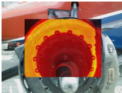
Figure 2: Front right carbon rotor, disk bell, and hub assembly
