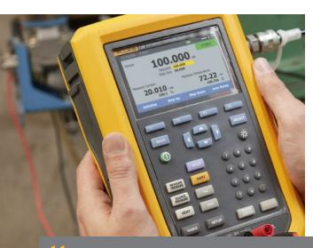
With the 729, we can automatically test multiple pressure points in one set up. We're able to get straight to the depression set point without having to bleed the pressure and pump it back up, which definitely makes us more efficient."
