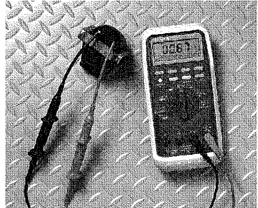
Figure 5. Ignition coil primary resistance
