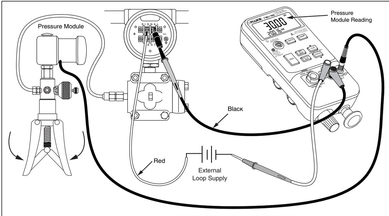
Figure 6. Pressure Module with External Pump
