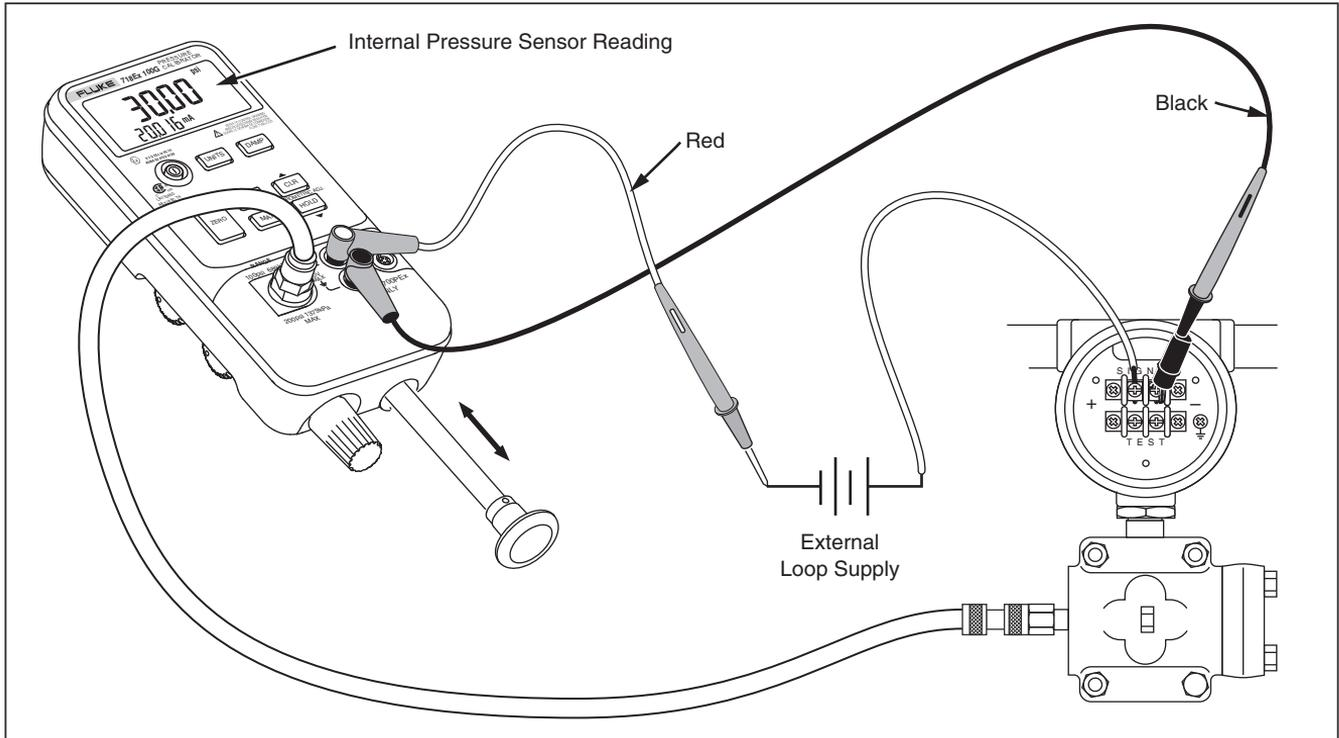
**Figure 4. Internal Pressure Sensor with Internal Pump**
