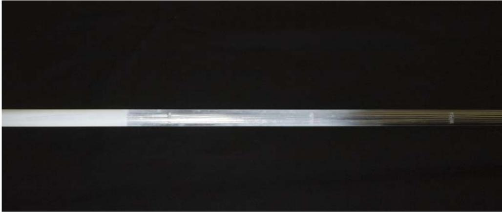
Figure 2: Devitrification of a fused-quartz glass sheath
