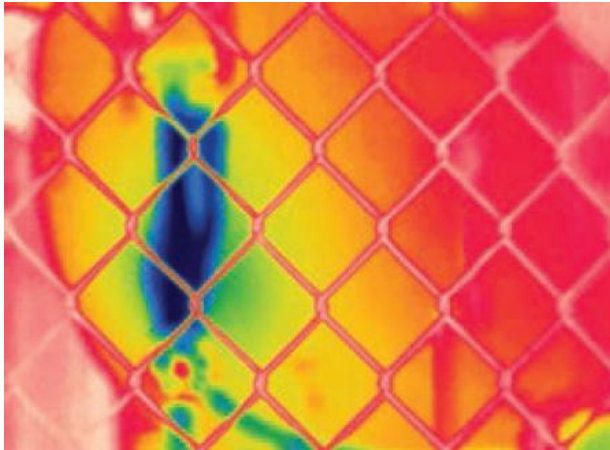
Figure 3: Passive auto focus systems often only capture near-field object
