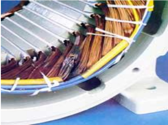
Figure A. Motor Insulation Burnt.
