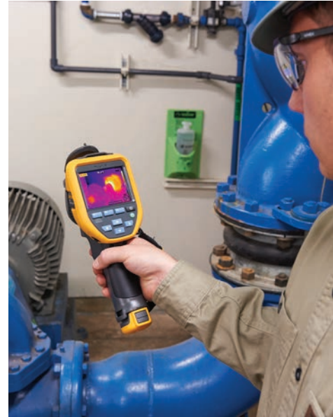
An engineer uses a Fluke TiS75 Infrared Camera to inspect a motor
