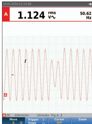
Trigger point is set to a point but due to the aberration on the leading edge in the second period, an additional trigger results in an unstable display.
